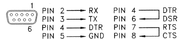
Figure-3 Connector Wiring Diagram
