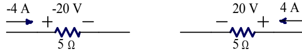
Figure 12. An illustration of how the passive sign convention is used. In both situations the flow of net positive current is from right to left. In both situations the right side of the resistor has the greater voltage in comparison to the left side.
