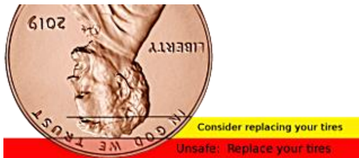
Figure 2, A penny can be used to measure the tread-depth of a tire. The penny is a common standard of measurement in this context.
