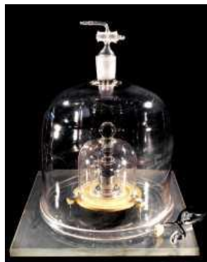
Figure 3, “Le Grand K,” The international prototype kilogram, under three nested bell jars, maintained by the Bureau International des Poids et Mesures, Sèvres, France [10].
